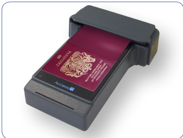
The OCR600e reading the MRZ and the passport chip in a single action
